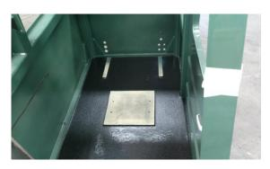
Drill Rigs Australia has found that cab floors are now easier to clean. Further, unlike cabs where rubber flooring is used, there is no issue with smell, build-up of dirt under the flooring or trip hazards from rubber mats swelling.
